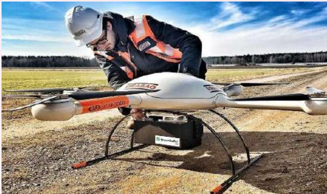
Figure 2: Drone Used for Site Survey and Monitoring
