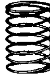
Closed-ended spring will tangle only under pressure
