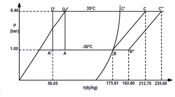
increases both the refrigeration effect as well as the work of compression.
