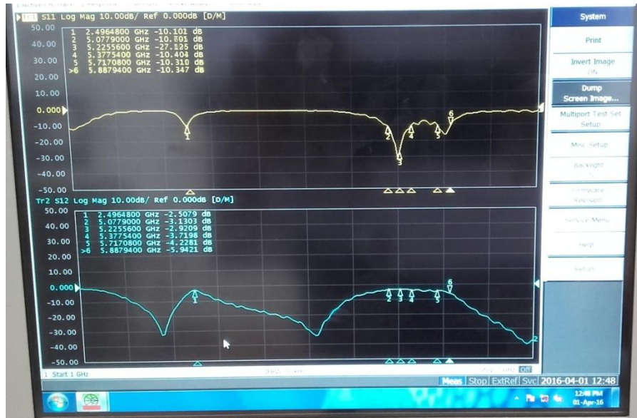
Figure 10(b) S_{11} and S_{21} versus frequency of the fabricated PSO based dual band filter for 2.5GHz and 5.3 GHz bands
